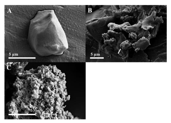
**Fig. 1.** Morphological analysis of starch hydrogel-based oral (SHO) vaccine. Field emission scanning electron microscopic (FESEM) specimen features: starch prior to forming hydrogel (A); synthesized hydrogel based on starch containing no antigen (an arrow defining porous structure) (B); SHO vaccine: starch-based hydrogel containing formalin-killed cells (*E. tarda* SU53) (C). The scale bar is 5 µm.
